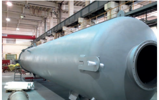
Quench column in the Wittenberg workshop rubber lining plant
